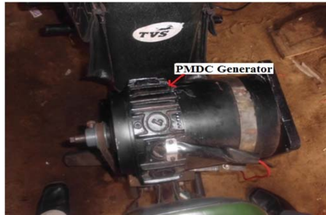
Figure 8: Experimental Setup PMDC generator
