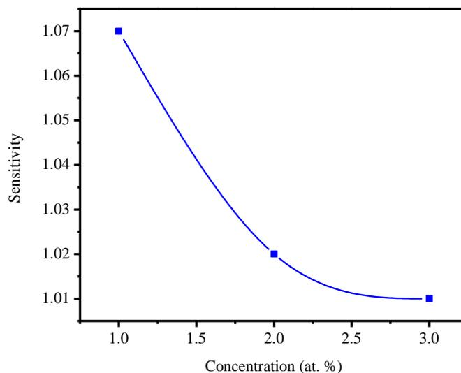
**Figure 10:** Variation in sensitivity with various concentration of CuO sensor, toward 100 ppm of ethanol.
