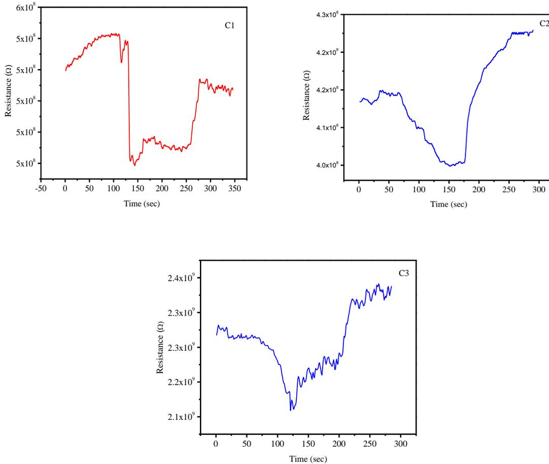
**Figure 9:** The response of CuO sensor prepared at various concentration, upon exposure to 100ppm of ethanol gas at room temperature.
