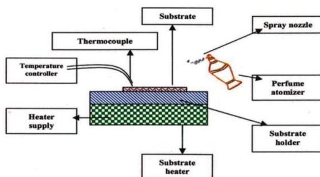
**Figure1:** Block diagram showing a simplified spray pyrolysis technique
