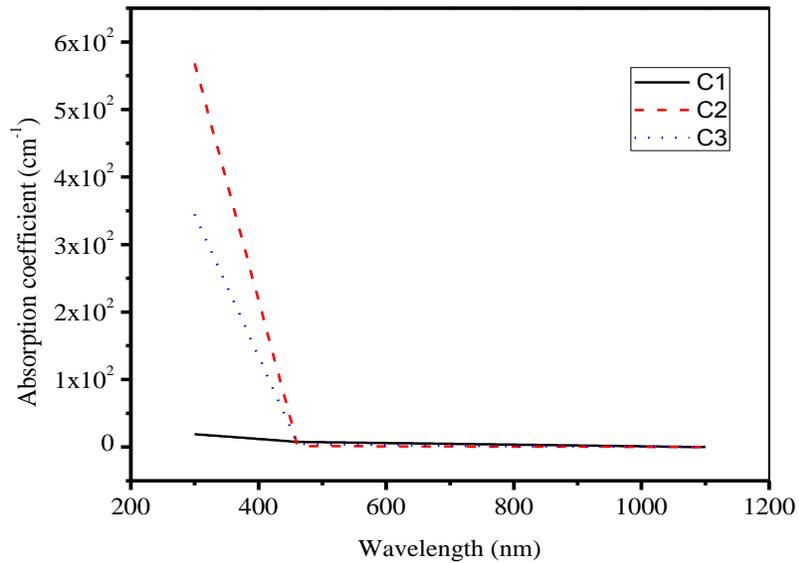
**Figure 4:** Linear absorption coefficient spectra of CuO thin films
