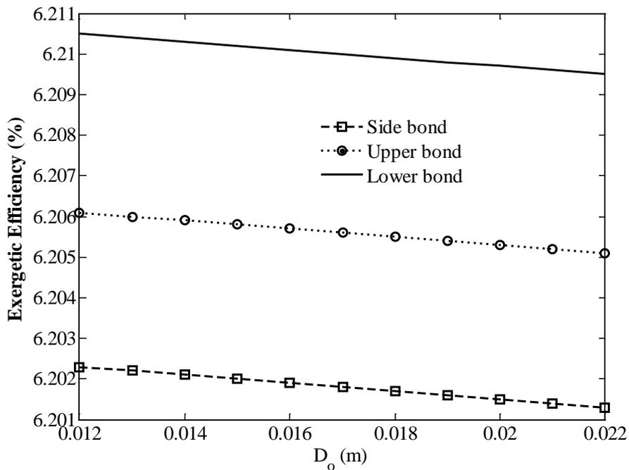
**Fig. 6.** The variations of the exergetic efficiencies versus the outer diameter of the riser tubes for the three models.
