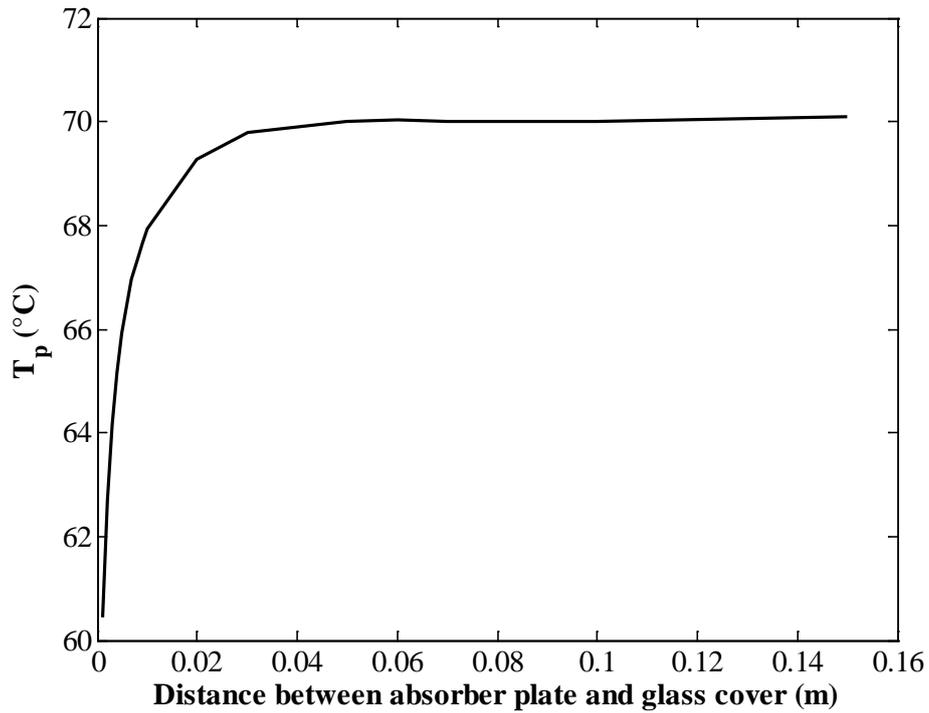
**Fig.8.** Variations of the absorber plate temperature versus the distance between absorber plate and glass cover.
