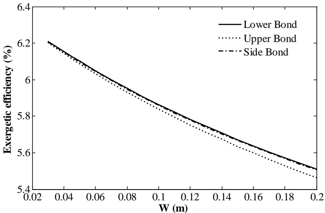
**Fig. 3.** The variations of the exergetic efficiencies versus the distance between riser tubes for the three models.
