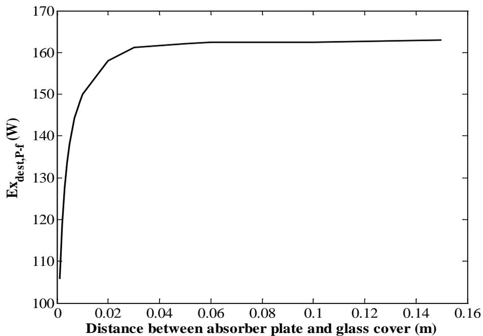
**Fig.12.** Variations of exergy destructing in the heat transfer process from absorber plate to working fluid versus the distance between absorber plate and glass cover.
