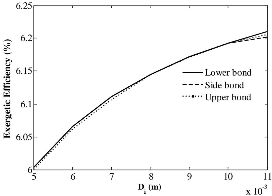
**Fig. 5.** The variations of the exergetic efficiencies versus the internal diameter of the riser tubes for the three models.
