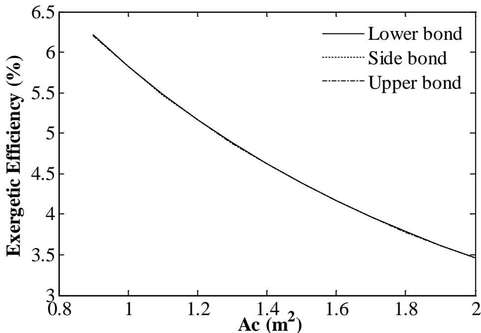
**Fig. 4.** The variations of the exergetic efficiencies versus the absorber plate area for the three models.
