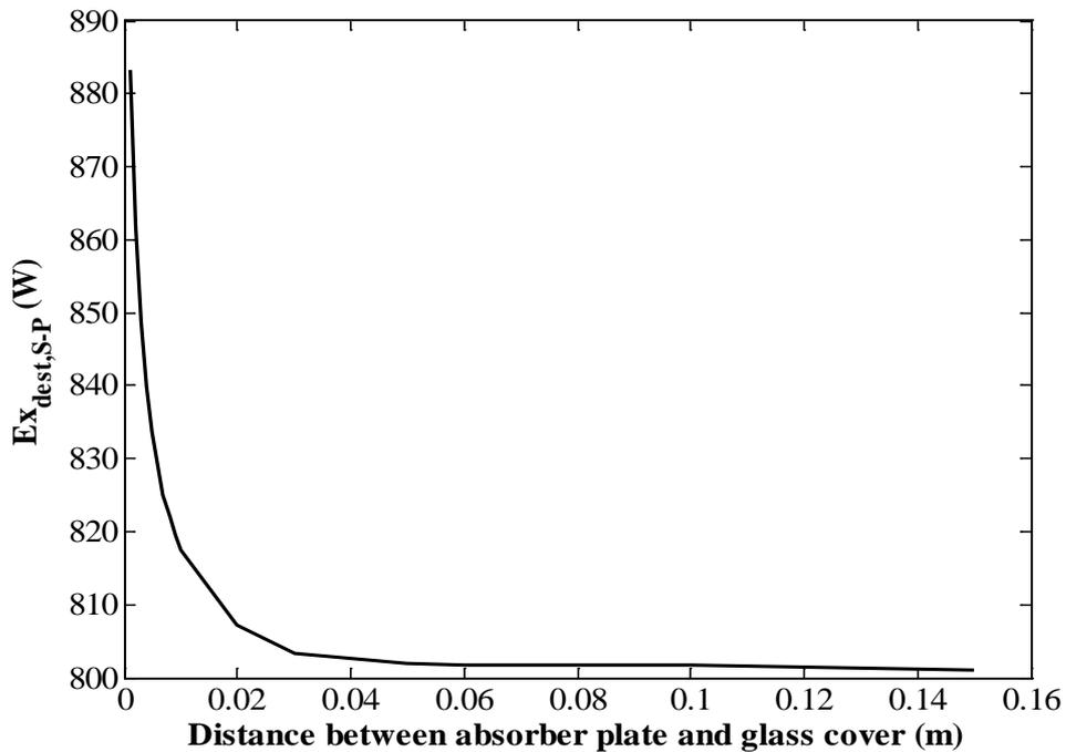
**Fig.10.** Variations of absorption exergy losses versus the distance between absorber plate and glass cover.
