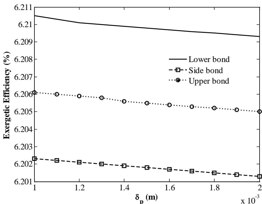
Fig. 7. The variations of the exergetic efficiencies versus the absorber plate thickness for the three models.
