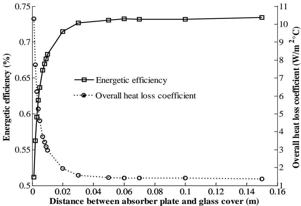
**Fig.9.** Variations of energetic efficiency and overall heat loss coefficient versus the distance between absorber plate and glass cover.
