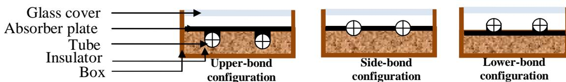
**Fig .1.** Various types of liquid flat-plate solar collector
