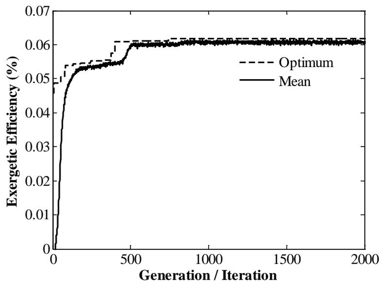
**Fig.2.** Convergence diagram for the optimization procedure
