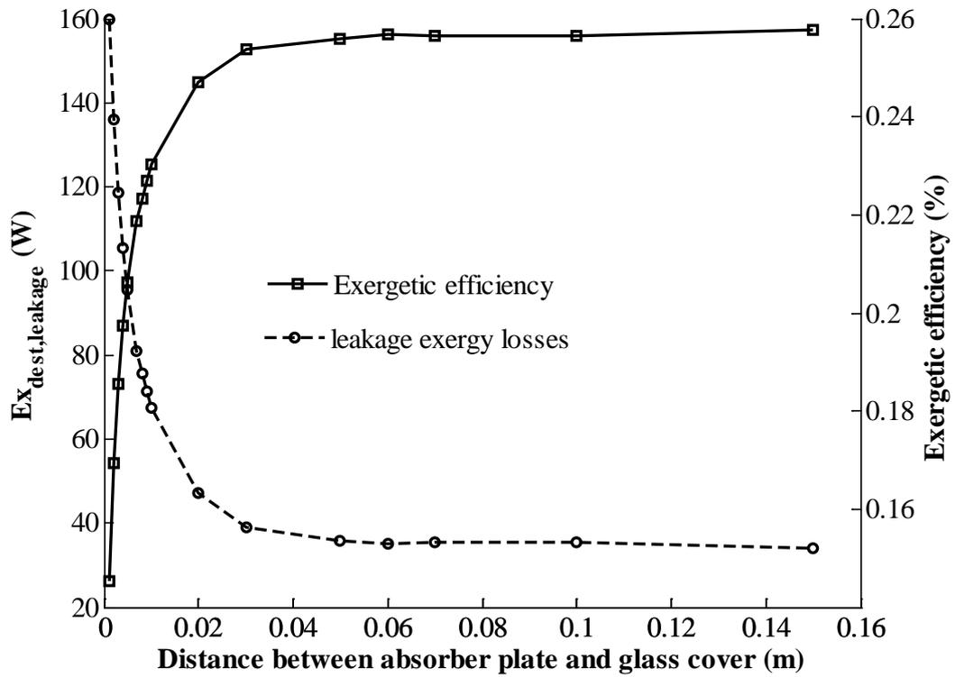
**Fig.11.** Variations of leakage exergy losses and exergetic efficiency versus the distance between absorber plate and glass cover
