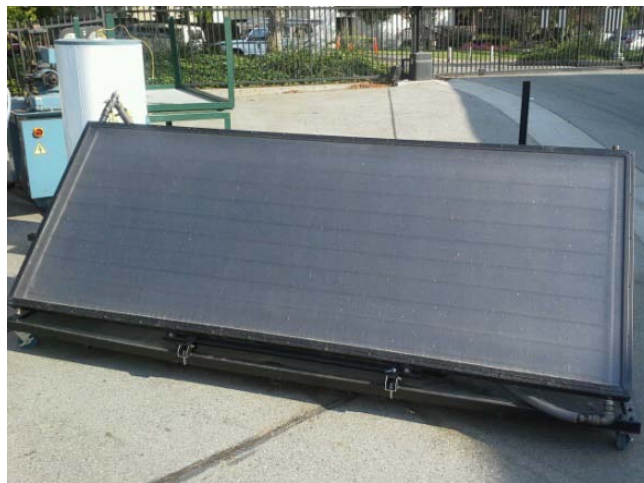
Figure 1. SUNEARTH solar collector test hardware
