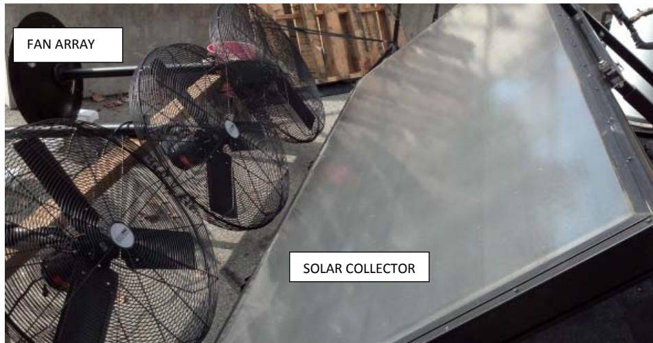
Figure 2. Test hardware showing proximity of forced convection simulation fans to solar collector test article
